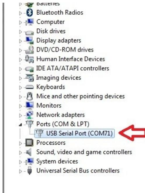
In Windows when you have drivers installed, you should see the relay board as USB Serial Port
